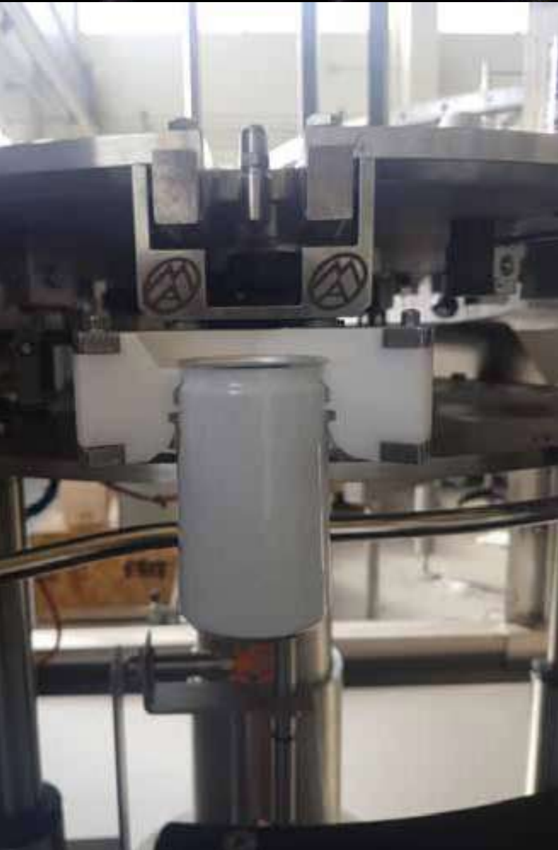
10.8.1, rotary rinser, no by gravity, no depal from the top, labelling of no printed cans before the rinsing
