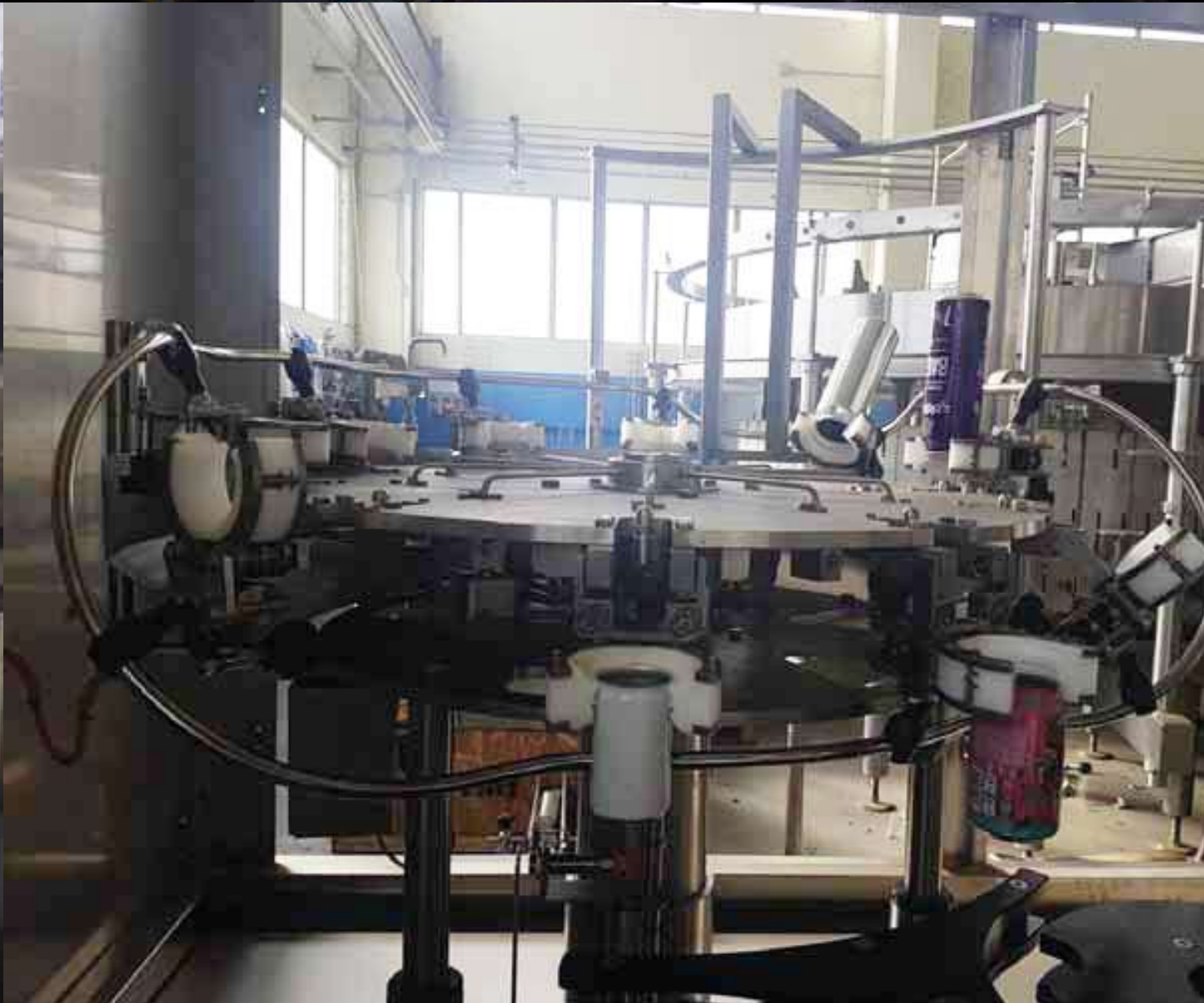
10.8.1, rotary rinser, no by gravity, no depal from the top, labelling of no printed cans before the rinsing
