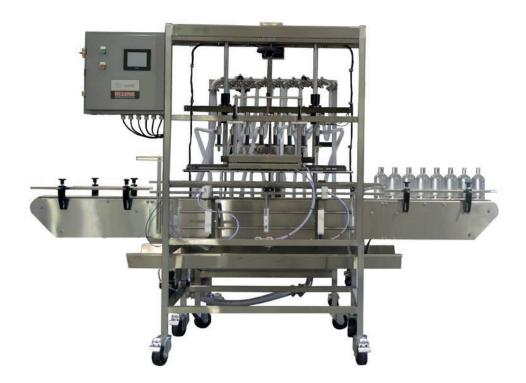
Based on a fill-to-level principle, the Model of Pressure Overflow Filler delivers a quantity of flowable liquid into the container until it reaches an adjustable fill height. Excess liquid then flows through the overflow vent back into a tank until the time cycle is complete and the filling head retracts.
